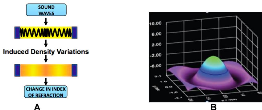
**Figure 1.** (A) Schematic of the Tunable Acoustic Gradient Lens principle. Sound waves cause the variation in liquid density and corresponding index of refraction that creates the lens effect. (B) Example aspheric wavefront profile
