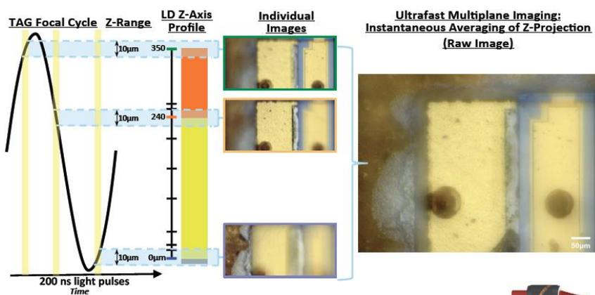
**Figure 3:** Multi-plane Imaging techniques: 2P microscopy, inspection, etc.
