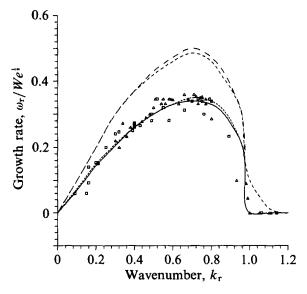
FIGURE 7 (Corrected). Comparisons of theories with experiments. Present results: Re = 3000, Re/Fr = 0, l = 10; ....., We = 0.0025, Q = 0, N = 0; ...., We = 0.0013, Q = 0.0013, N = 0.018; ...., We = 0.0025, Q = 0.0013, N = 0.018...., Rayleigh;  $\triangle$ , Goedde & Yuen;  $\square$ , Donnelly & Glaberson.
