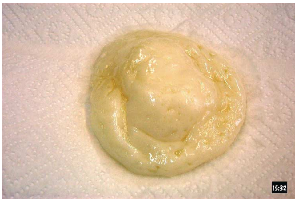
Fig 5. A chemical gel trapping an oil-in-water emulsion.
