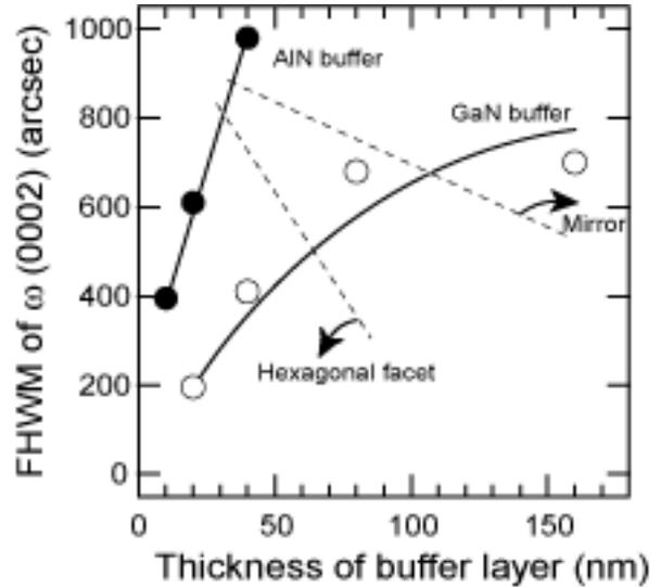
Figure 19. The FWHM value of  $\omega$  (0002) for 1  $\mu\text{m}$  HT-GaN films deposited on AlN (closed circles) and GaN (open circles) buffer layers with the thicknesses in the figure. The buffer layers were annealed for 10min under the optimum ambient. Their polarity changed as indicated by the surface morphology, and the polarity conversion occurred drastically in the case of the AlN buffer layer.
