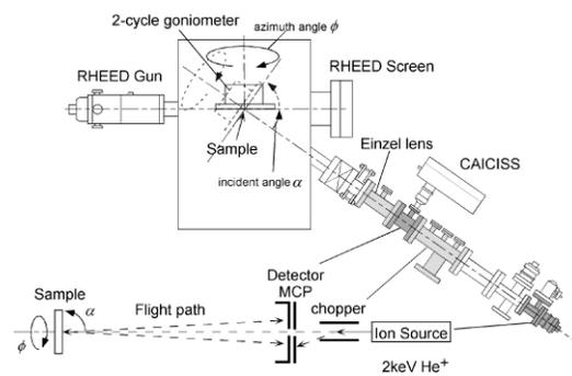
Figure 3. Schematic illustration of CAICISS apparatus with a chamber and block diagram. The incident and azimuth angles of the ion beam can be altered by moving the sample holder, which is equipped with a heater.
