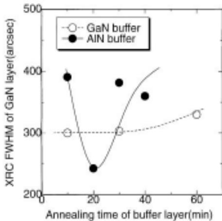
Figure 18. FWHM of  $\omega$  (0002) for HT-GaN films deposited on GaN (open circles) and AlN (closed circles) buffer layers with the same thickness, when the buffer layers were annealed for the times shown in the figure. The conditions for obtaining better quality HT-GaN material are wider with GaN buffer layers [127].
