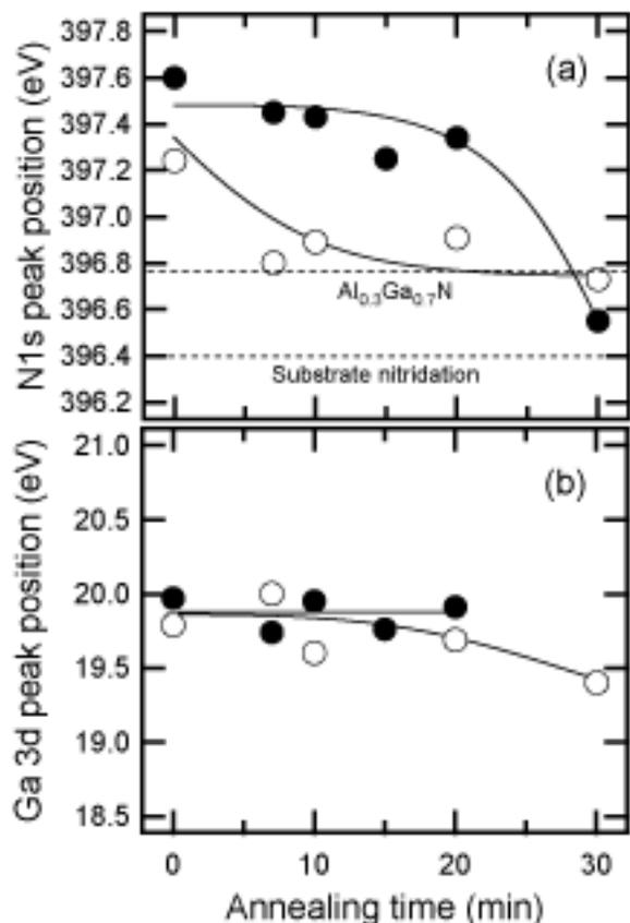
Figure 14. Dependence of (a) N1s and (b) Ga 3d peak positions for a 20-nm-thickness GaN buffer layer on H<sub>2</sub> cleaned (open circles) and nitrided (closed circles) sapphire substrates on the annealing time under the N<sub>2</sub> and H<sub>2</sub> mixed ambient. The positions were detected by XPS analysis. [after Ref. 117] The sample on the nitrided substrate evaporated completely, and AlGa<sub>0.3</sub>N was formed at the interface between the sample and the non-nitrided substrate.
