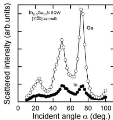
Figure 7. Incident angle dependence of Ga and In scattered intensity at the  $[11\bar{2}0]$  azimuth for  $\text{In}_{0.5}\text{Ga}_{0.5}\text{N}$  SQW. Variation of both the Ga and In signals indicates +c polarity judging from the CAICISS results on ZnO bulk given in Fig. 5. Indium atoms incorporated into an  $\text{In}_x\text{Ga}_{1-x}\text{N}$  SQW were found to occupy substitutional Ga sites. [52]]
